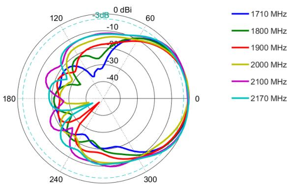
**Elevation (Side View): 1710 – 2170 MHz**
