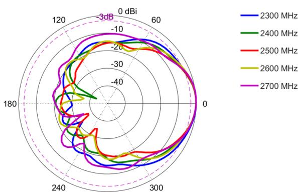
**Elevation (Side View): 2300 – 2700 MHz**
